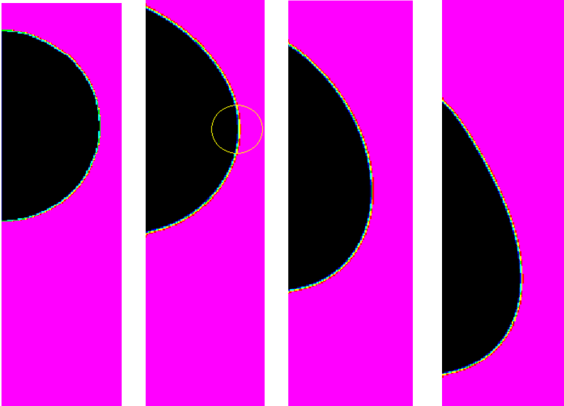
Figure 4. Flow of droplet down wall. Profile across interface of circled area shown in next figure.
